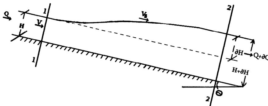
Fig. 1. Scheme of calculation of debris flow continuous wave with constant discharge along the way.
