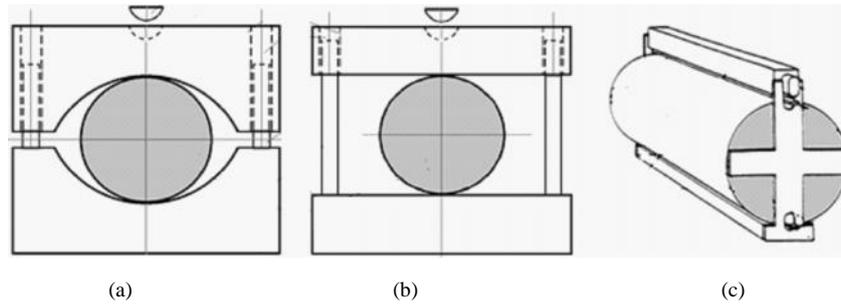
Fig. 2. The schemes of apparatus of ISRM (a), of ASTM (b) and BS EN (c) Standard Test Methods for Splitting Tensile Strength of Intact Rock Core Specimen.
