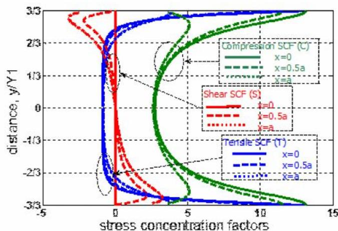
Fig. 4. Principal normal tensile (T), compressive (C) and shear (S) stress concentration factors (SCF), on the vertical diameter ( $x=0$ ;  $0 < y/R_1 < 1$ ), and on the nearby chordal sections ( $x=0.5a$ ) and ( $x=a$ ).
