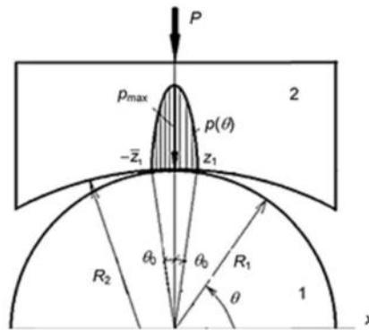
Fig. 3. Compression of a cylindrical specimen between curved jaws.  $z_1$  and  $-\bar{z}_1$  are the boundary points of the contact surface.
