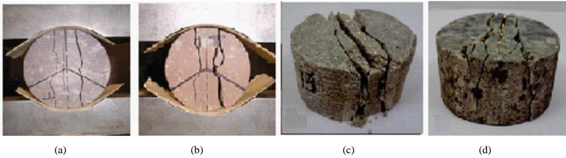
**Fig. 1.** Examples of chordal fracture in Brazilian test of Yucca Mountain Tuffs (a,b) (From Daemen, et al. [7], sandstone (c) and granite (d) specimens (From Basu, et al. [30] ).
