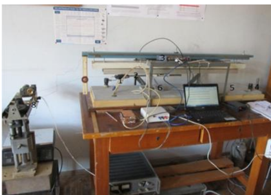
Fig. 2. Experiments on the Burridge-Knopoff (BK) model with registration of accelerations, acoustic emissions and pulling force: 1. pulling force measuring dynamometer; 2. upper (movable) platform; 3. Picoscope; 4. acoustic sensor; 5. immovable (static) plate; 6. movable (slidable) plate; 7. power supply; 8. pulling system.
