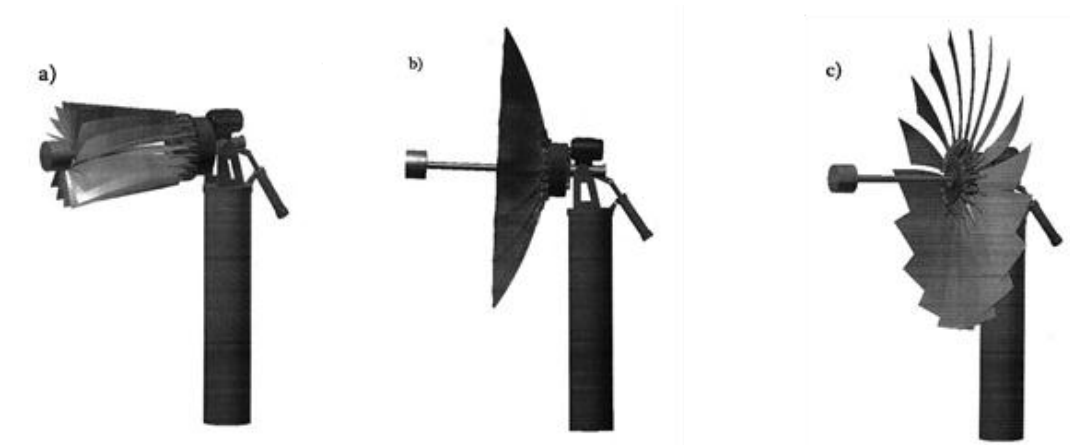
Fig. 1. The Spatial diagram of stages of wind and solar power equipment: a) the device in folded position; b) the device in the position of solar reflector; c) the device in the position of wind turbine
