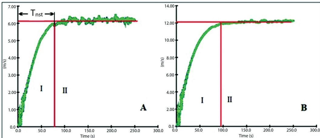
**Fig 2.** The variability of the oncoming air flow velocity in time, when the first carriage of a train (its length is 80 m) is in distance of 130 m from the place of a joint between the station and the tunnel: A – nature of variability of the oncoming air flow; B – nature of variability of the velocity in the annular space; I – non-stationary phase; II – stationary phase; the time of modelling – 600 s;  $T_{nst}$  – duration of the non-stationary phase, s.
