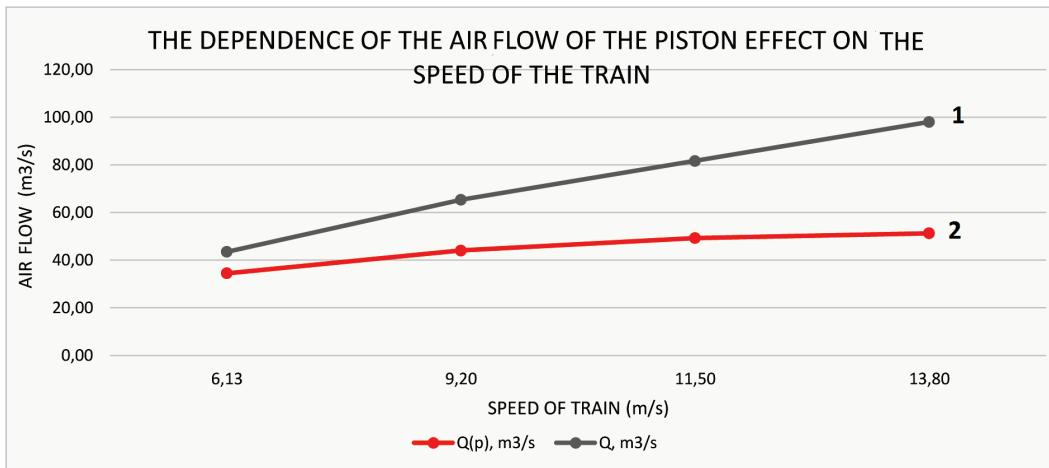
**Fig. 3.** The rate of air flow, induced by piston effect, depending on a train's speed:
