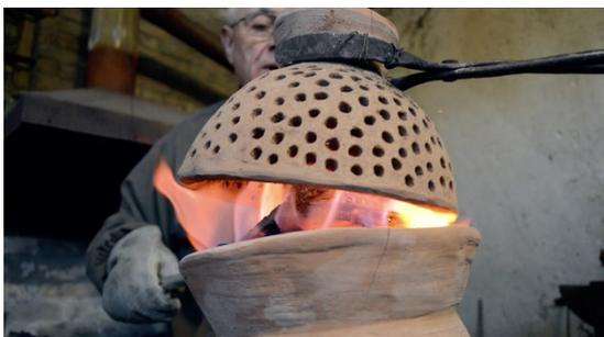
**Fig. 6.** Soldering of the Goblet copy with the analogue of Kvatskhela muffle.
