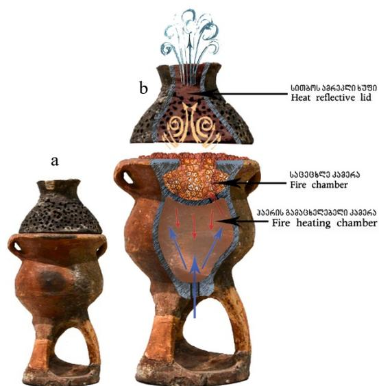
Fig. 5. a) The layer of substantial solder revealed on the goblet; b) Operating scheme of Kvatskhela muffle.
