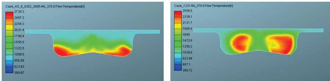
**Fig. 1.** The instantaneous local values of the temperature (K) in the burning chamber of the hydrogen (on the left) and traditional (on the right) diesels, when the angle of rotation of the crank-shaft  $\varphi=370^0$  ( $m_{ds}=0.24$  g/cycle,  $m_{H2}=0.085$  g/cycle).
