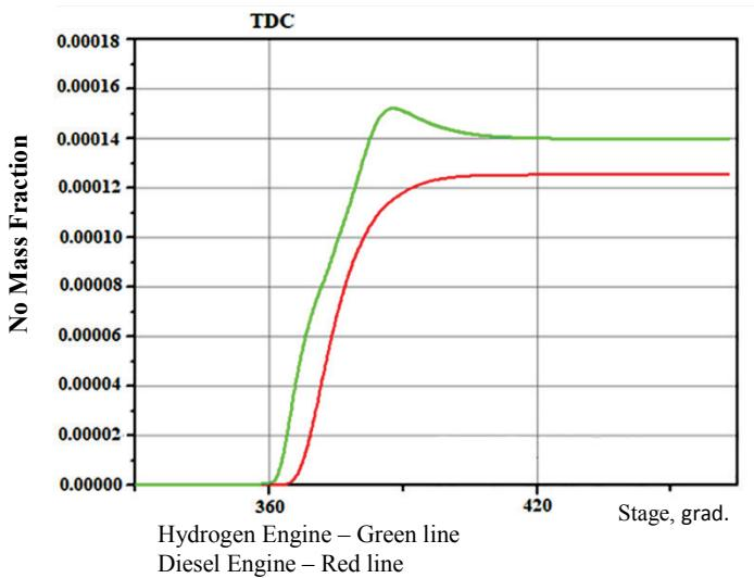
**Fig. 3.** Change of the nitric oxides total concentration depending on the angle of rotation of the crankshaft in the hydrogen (1) and traditional (2) diesels.
