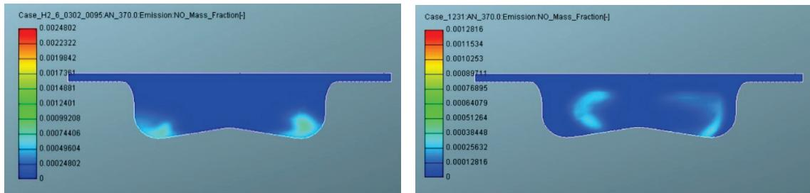
**Fig. 2.** The instantaneous local values of the nitric oxides concentrations (mass portion) in the burning chamber of the hydrogen (on the left) and traditional (on the right) diesels, when the angle of rotation of the crank-shaft  $\varphi=370^0$  ( $m_{ds}=0.24$  g/cycle,  $m_{H2}=0.085$  g/cycle).
