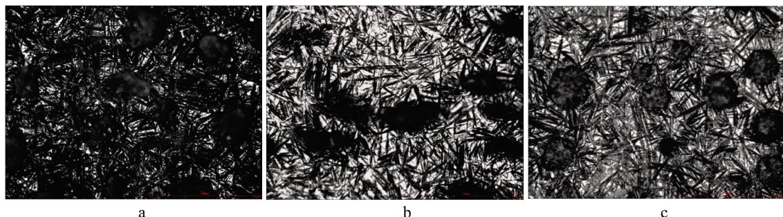
**Fig. 3.** Microstructures (X400) of isothermal quenched (at the  $280^\circ\text{C}$ ) ductile iron, depending on the degree of plastic deformation: a)  $\epsilon \approx 30\%$ , b) Ingot, c)  $\epsilon \approx 65\%$ .
