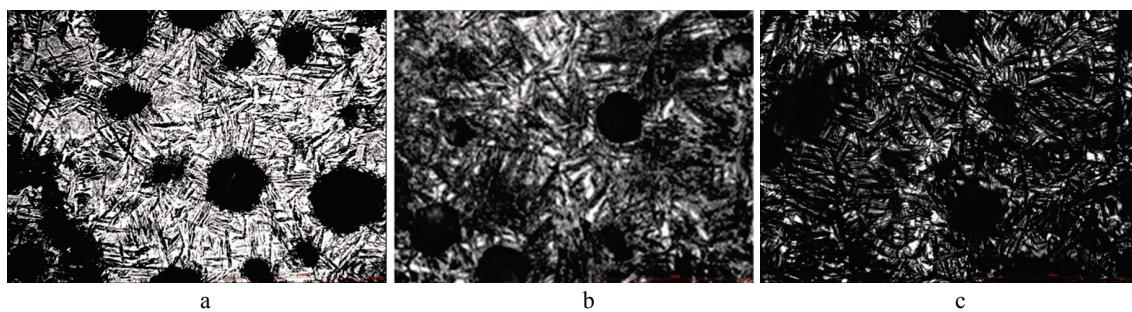
**Fig. 4.** Microstructures (X400) of isothermally quenched (at the  $400^\circ\text{C}$ ) ductile iron, depending on the austenitization time: a) 30 min, b) 45 min, c) 60 min.
