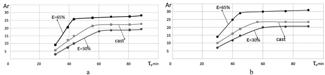
**Fig. 2.** Influence of austenization time on the amount of retained austenite after isothermal treatment during 30 minutes at the temperatures: a)  $280^\circ\text{C}$  and b)  $400^\circ\text{C}$ .
