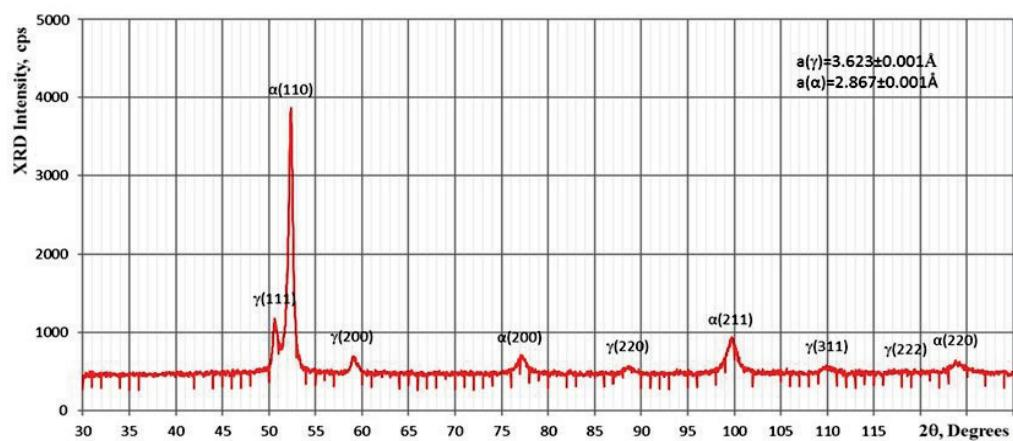
**Fig. 1.** XRD diffractogram of bainitic ductile iron.
