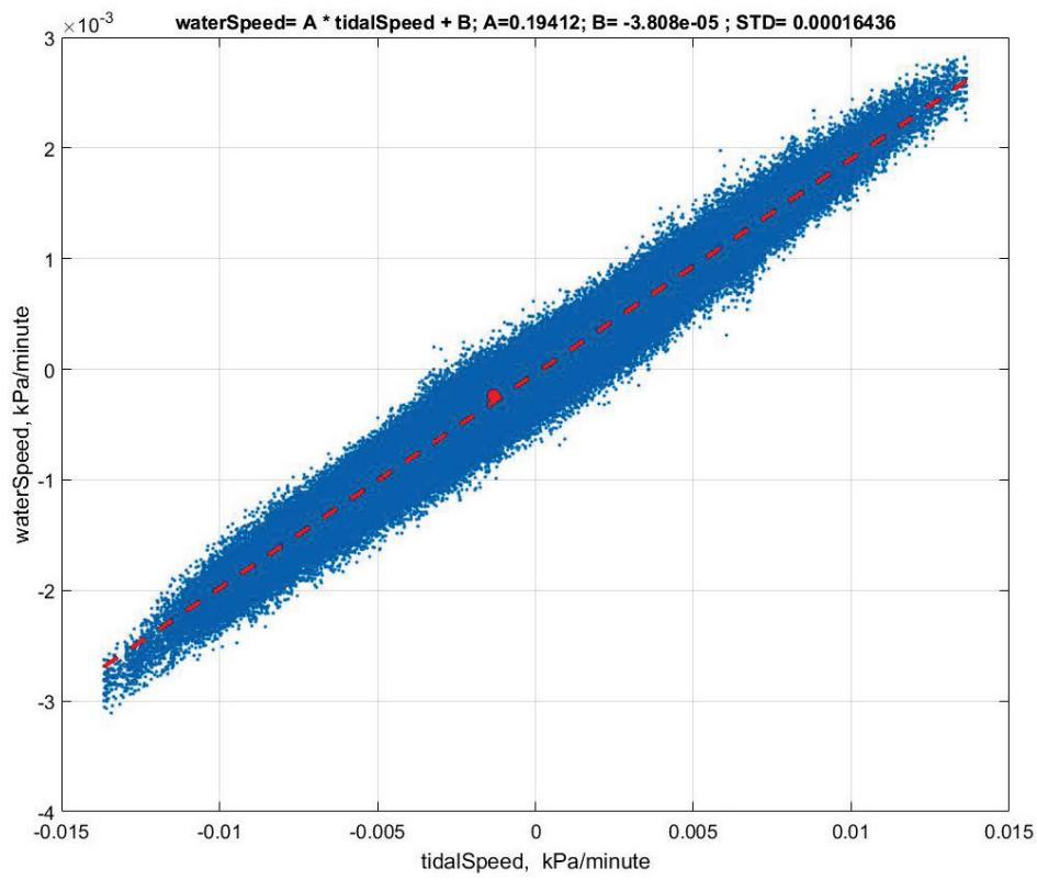
**Fig. 1a.** On X axis is the tidal force change (kPa) and on Y axis the water level change (kPa).
