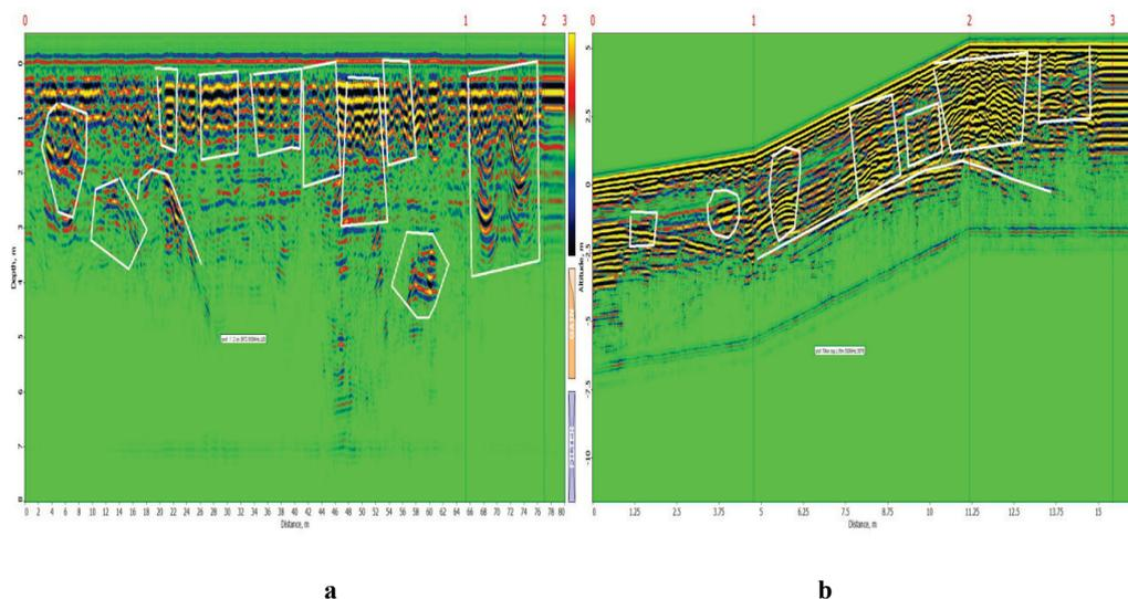
**Fig. 3.** a) The first ellipse-shaped profile (Profile 1cir, the length – 80 m).
