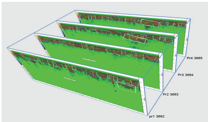
**Fig. 4.** A spatial image of parallel profiles Pr.1, Pr.2, Pr.3, Pr.4 in the *Area-A* (see Fig.1) processed by the similar amplification option. Linear radio images are revealed at 2-3 m depths on all four parallel profiles.
