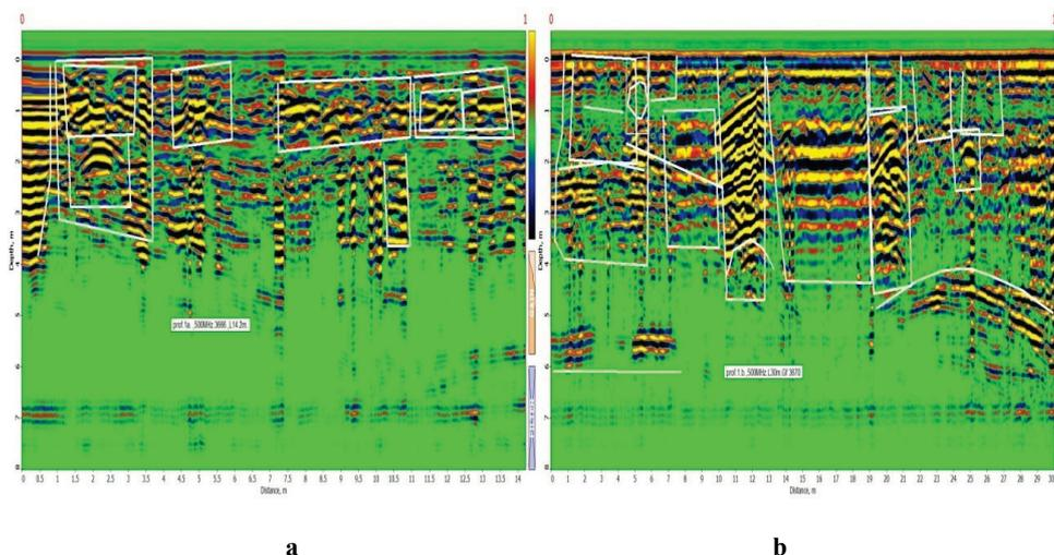
Fig. 2. a) The georadiolocation section of the profile 1A was obtained by 500 MHz antenna on a 14 m long and 7 m penetration depth profile. Radio images of linear tube-like objects were obtained from parallel profiles 2A, 3A, 4A.
