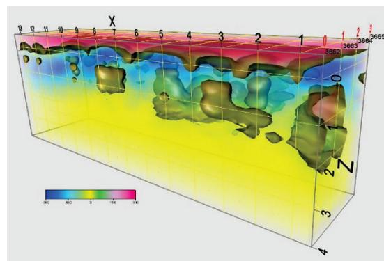
**Fig. 5.** A symmetric arrangement of near-surface probable voids on the parallel profiles Pr.1, Pr.2, Pr.3, Pr.4 in the *Area-A* (see Fig. 1). The profile images were produced using software VOXLER 3D compatible to PRISM 2.5.
