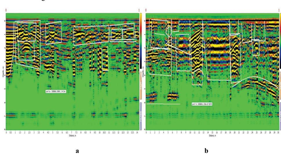
**Fig. 2.** a) The georadiolocation section of the profile 1A was obtained by 500 MHz antenna on a 14 m long and 7 m penetration depth profile. Radio images of linear tube-like objects were obtained from parallel profiles 2A, 3A, 4A.
