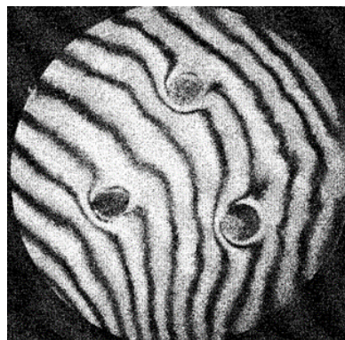
Fig. 1. One of the interferograms from the entire observation cycle (462 hrs.) in a cement matrix with three large granites in the free state for observation time of 114 hrs.
