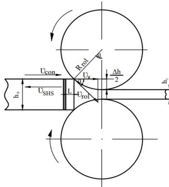
Fig. Diagram of SHS-electric rolling.
