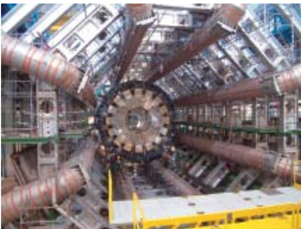
Fig. 13. The barrel has arrived to its final position at the ATLAS centre
