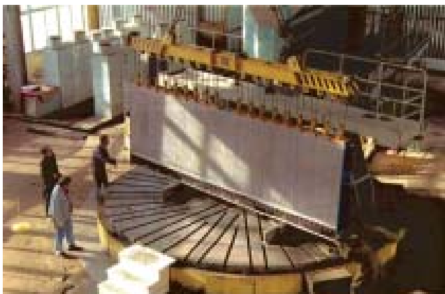
Fig. 5. April 1996. ATLAS Module 0 at the 6-meter chuck plate of the vertical boring and turning machine, JINR, Laboratory of Nuclear Problems.
