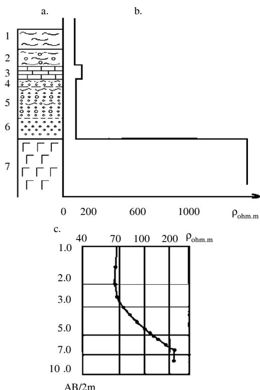
Fig. 1. a – Geologic section: 1. light brown clay; 2. light brown loamy clay, 3. carbonates, 4. brown loam, 5. dark brown loam with sand inclusions, 6. volcanic ash, 7. basalts. b – resistivity distribution with depth according to parametric measurements, c - vertical electric sounding (VES) curve.
