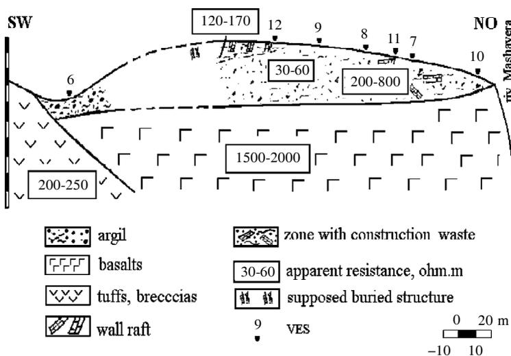
Fig. 2. Geoelectric section I in the area of old settlement.
