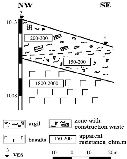
Fig. 3b. Geoelectric section III, the territory of old settlement
