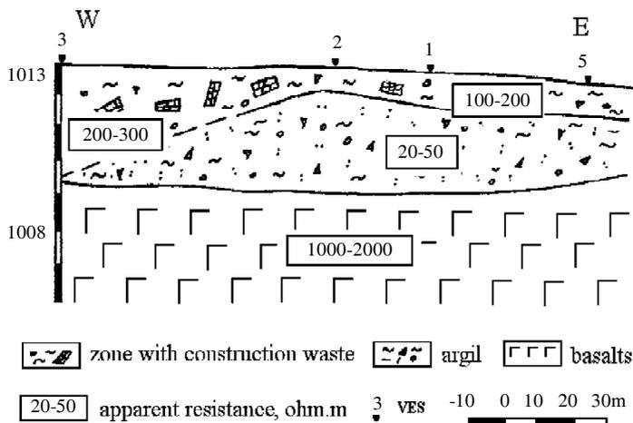
Fig. 3a. Geoelectric section II, the territory of old settlement.
