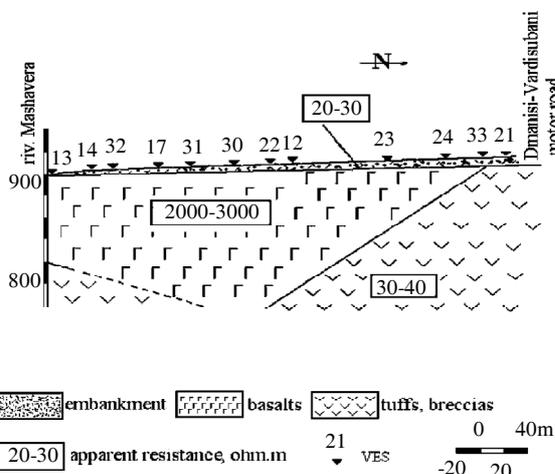
Fig. 4. Geoelectric section, the territory between riv. Mashavera and motor road.
