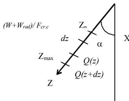
Fig. 2. The scheme of heat flows in the elements of cryocondenser
