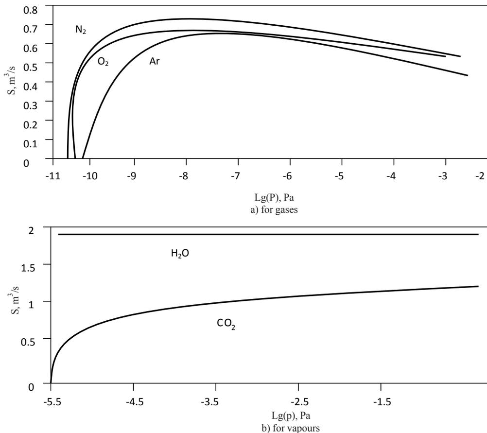
Fig. 3. Pumping speed dependence action on pressure
