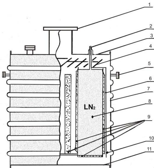
Fig. 1. General view of the cryosorption pump CSP-0.25D
