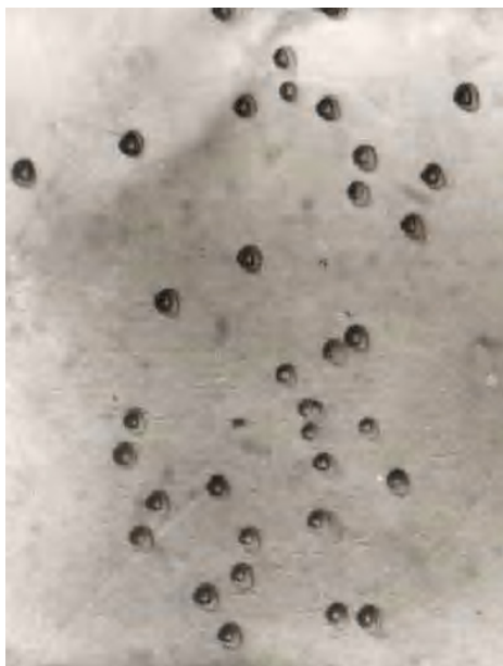
Fig.1. Microstructure of monocrystalline \text{Si}_{99.97}\text{Ge}_{0.03}:\text{As} solute solution a) \text{Si}_{99.97}\text{Ge}_{0.03}:\text{As} ( 1 \cdot 10^{16} \text{ cm}^{-3} ) b) \text{Si}_{99.97}\text{Ge}_{0.03}:\text{As} ( 5 \cdot 10^{19} \text{ cm}^{-3} )
