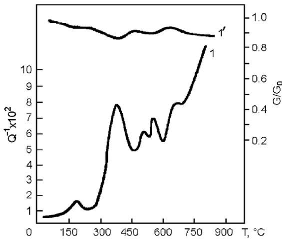
Fig. 1. Temperature dependence of internal friction (1) and shear modulus (1') of ceramic-metal Si<sub>0.8</sub>Ge<sub>0.2</sub>:P alloys
