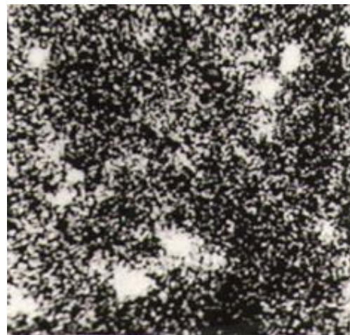
Fig. 4. Electronic micrography of the oxidized surface of ( T=1100^{\circ}\text{C} the scanning area - 100\times 100\text{ mkm} ) a - In absorbed electrons b - In x-ray Ce - L_{\alpha} radiation
