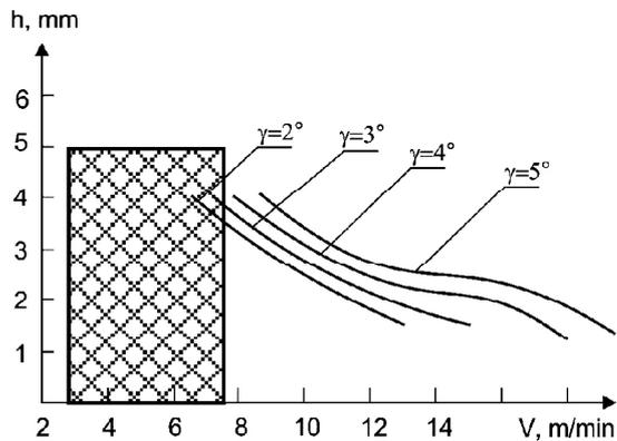
Fig. 4. Dependence of drawing velocity of a copper billet on its cross-section and  $\gamma$ -angle ( $\alpha = 30^\circ$ ,  $K = 2.6 \cdot 10^{-5}$ ;  $x_0 = 7 \cdot 10^3$ ;  $R = 0.21$  m)
