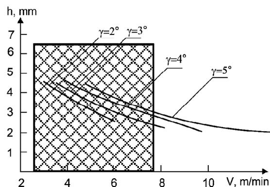
Fig. 3. Dependence of drawing velocity of a steel billet on its cross-section and  $\gamma$ -angle (for steel 45  $\alpha=30^\circ$ ,  $K = 0.8 \cdot 10^{-5}$ ;  $x_0 = 3 \cdot 10^3$ ;  $R = 0.21$  m)
