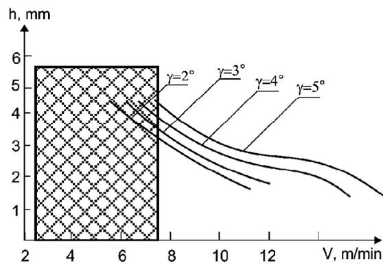
Fig. 5. Dependence of drawing velocity of an aluminium billet on its cross-section and  $\gamma$ -angle ( $\alpha = 30^\circ$ ,  $K = 2.8 \cdot 10^{-5}$ ;  $x_0 = 9 \cdot 10^3$ ;  $R = 0.21$  m)
