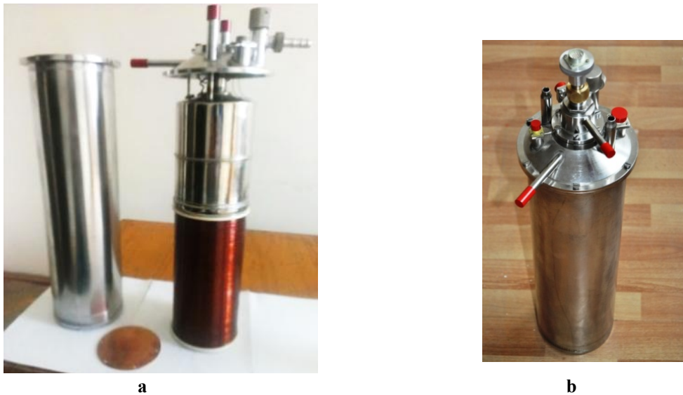
Fig. 3. a) Cryostat with undressed case; b) General view of cryostat.
